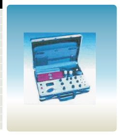
C201 is Battery / Mains operated Micro controller based instrument in briefcase for estimation of PH, Conductivity, TDS, MV, Dissolved Oxygen (D.O.) and temperature measurement in water, waste water and biological applications, pH meter is used for measurement. Measurement are displayed by a 20 x 4 digit alpha-numeric LCD.
