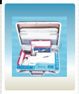
C203 is Battery /Mains operated micro controller based instrument in briefcase for estimation for PH, Conductivity, TDS, MV, Dissolved Oxygen (D.O.), Turbidity, Colori and Temperature measurement in water, waste water and biological applications PH meter is used for measurement. Measurements are displayed in 20 x 4 alpha-numeric LCD.
